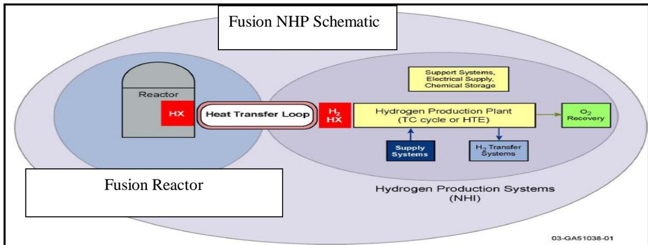
**Figure 2:** A nuclear hydrogen facility clearly showing the heat exchangers and heat transfer loops. At this conceptual level, the heat source is a Fusion reactor (“Generation V”) but can also be a high-temperature Fission (“Generation IV”) reactor. (Graphic adapted from Sherman 2006).
