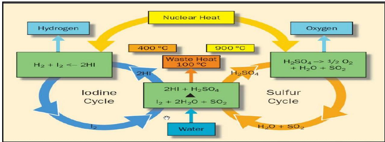
**Figure 1:** Concept of the sulphur-iodine S-I thermochemical cycle. Heat required can be supplied from either a fusion or a fission reactor.
